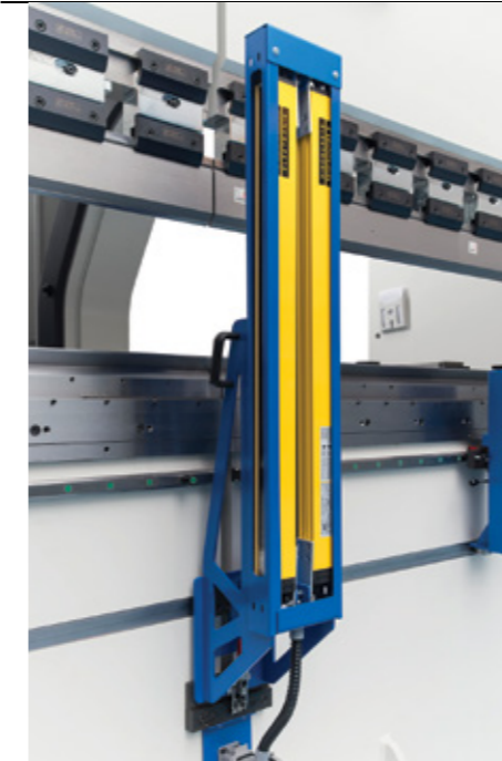
TI 1 Safety system Barriers
