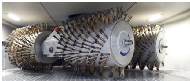
Brush for removing oxide layer
